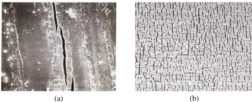
Fig. 19.8 (a) MIO breach in inner insulation and (b) ESC in outer insulation
