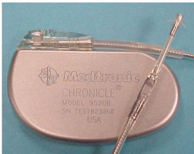
Fig. 19.14 Photograph of the Chronicle Implantable Hemodynamic Monitor and pressure sensor on the lead
